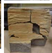
Fig 2 100mm cut on Zirconia under 5m of water
